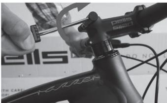
5. Now check that the headset (steering) is positioned correctly. This is easy to tell: the handlebar must turn freely and smoothly, and the steering must be free of play. You can detect any play by standing over the frame, pressing the front brake with your left hand, gripping the top cup of the headset with your right hand and moving backwards and forwards with your right hand. You should not feel any play (the fork is neither knocking nor loose in the headset).
