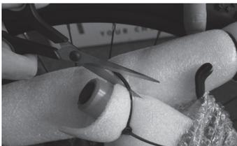
2. Using a Stanley knife or scissors, carefully remove the foam padding and other packing material. Be careful not to scratch the frame.
