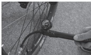
**Checking the shock pressure**
