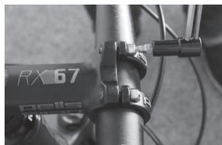
4. Align the handlebar so that the stem and front wheel are in line (if the stem cannot be turned, loosen the two bolts on the side of the stem slightly). The best way to align the stem is to stand over the frame, hold the front wheel with your knees, and centre the stem with both hands.
