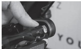
Once you have identified the correct pedal for each side, you can start attaching them. We recommend greasing the threads of both pedals with petroleum jelly. This is important if you don't want the pedals to harden in the threads over time or after they have been exposed to the elements.
